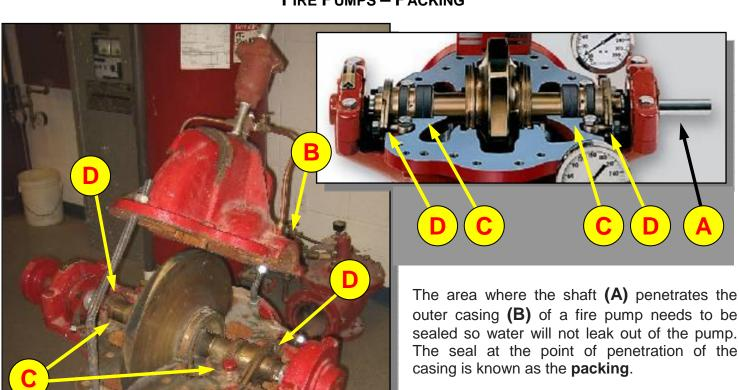
outer casing (B) of a fire pump needs to be sealed so water will not leak out of the pump. The seal at the point of penetration of the
