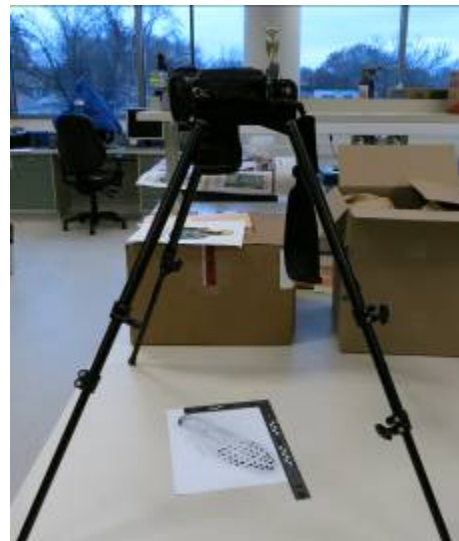
Figure 2: This is the position a photograph should be taken at. Using a tripod is best because it reduces shake and ensures you are directly over the impression. You can check the position of the camera from the side or using a level.
