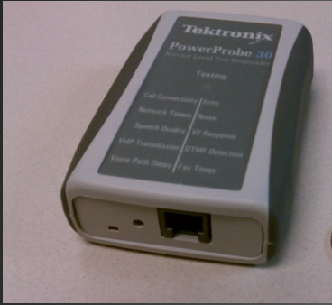
Device at PSAP (Tektronix PP30) used for MOS Score Calculation and other quality measurements.
