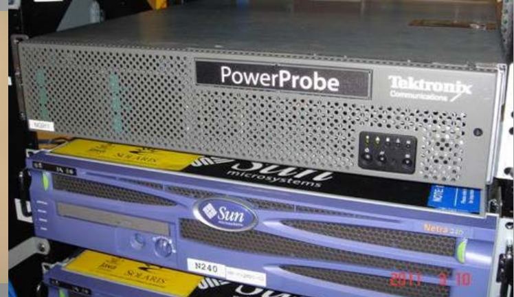
Centrally located Active Testing Device (Tektronix PP600) Makes and Measures Test Calls to PSAP
