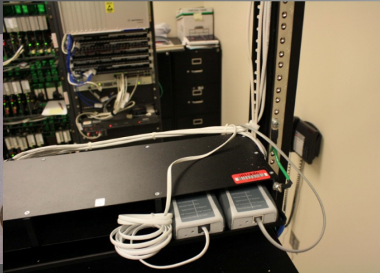
Device at PSAP (Tektronix PP30) used for MOS Score Calculation and other quality measurements.
