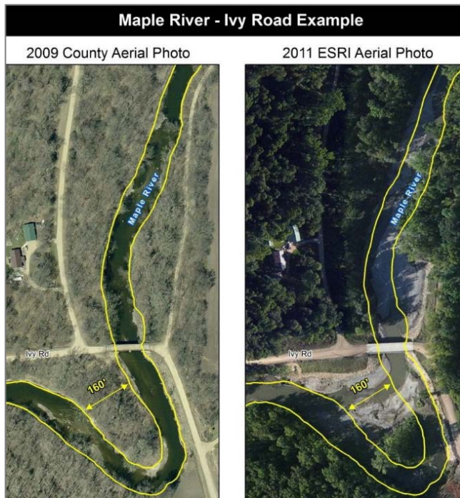
Figure 61. Example of Streambank erosion before event and after restoration.
