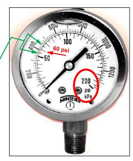
Each and every gauge on a system does not have to be tested for accuracy or calibrated. Comparing the reading of the tested or calibrated gauge to other gauges on the sprinkler system is permissible. For example, pressure gauges on systems that are installed in similar positions and elevations (e.g. on an adjacent riser) that show similar readings are acceptable.
